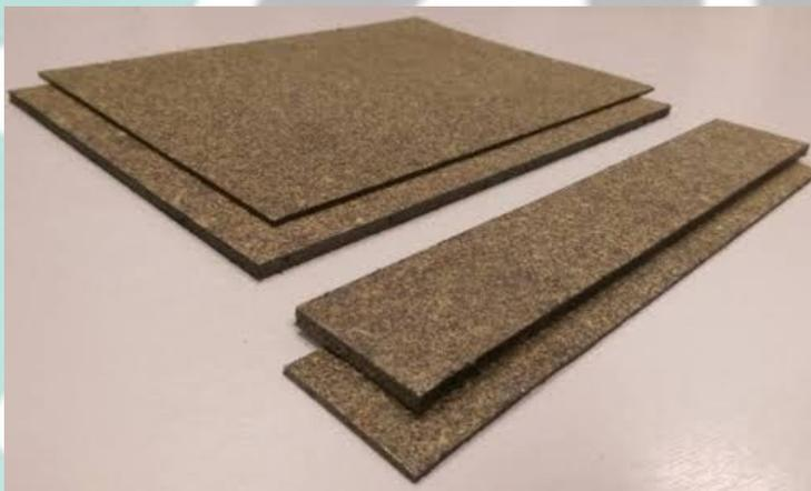
Millboard sheets are non-asbestos and non-ceramic fibre. They are for high temperature applications in centrifugal casting. These fibre boards possess high temperature capability, in excess of  $1,000^{\circ}\text{C}$ , and low thermal conductivity (K value), less than  $0.1 \text{ W/mK}$ , making them the first choice for thermal insulation applications.
